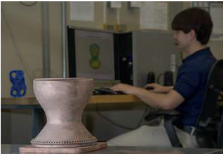
Figure 3.3. NASA's First Full-Scale Copper Rocket Part [85]
